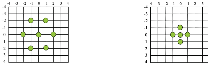
(a) Large hexagonal search pattern (LHSP) (b) Small hexagonal search pattern (SHSP)
