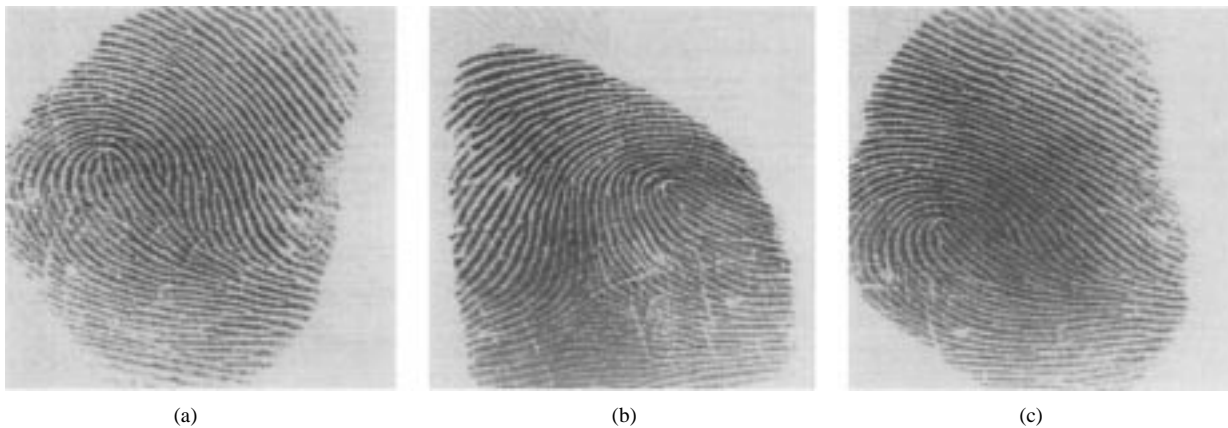
Fig. 17. Fingerprint images captured with a scanner manufactured by Digital Biometrics. The size of these images is 640 \times 480 ; all three images are from the same individual's finger.
