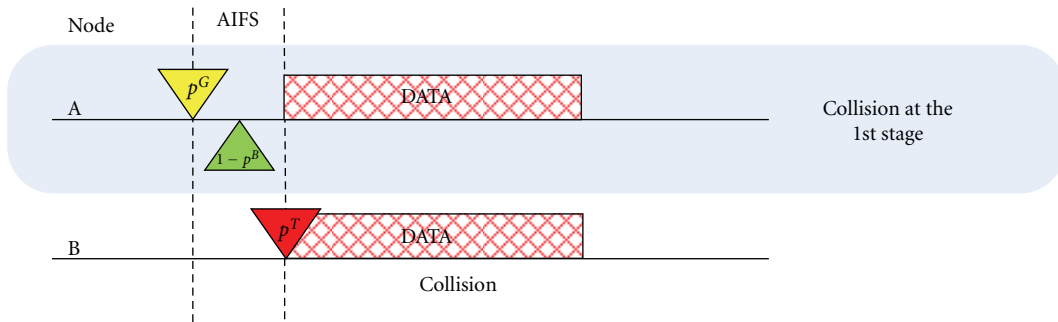
FIGURE 4: Diagram illustrating the action sequences related to a collision at the 1st stage.
