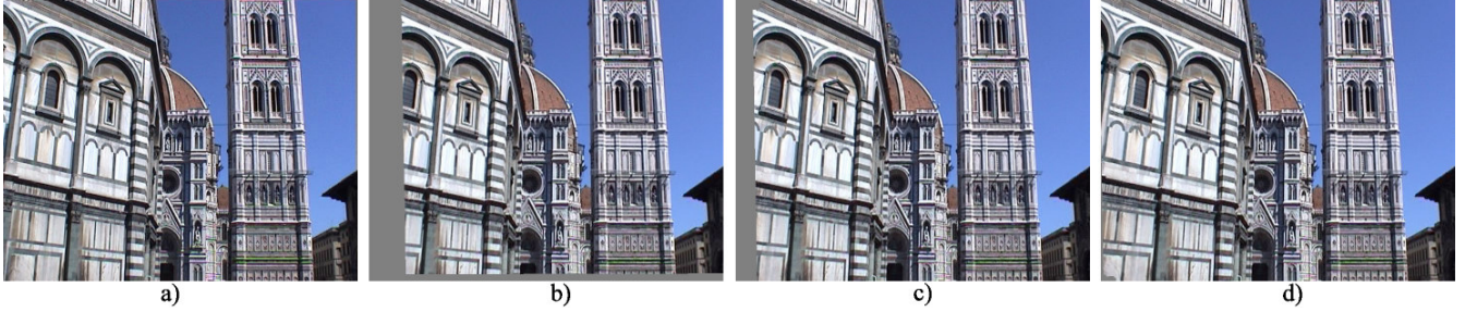
Fig. 3. Padding of pixels with additional frames: a) original left view of the sequence "Dome", b) virtual right view, only rendered with the closest view of the camera path, c) virtual right view using 30 and d) 62 frames of the original sequence.
