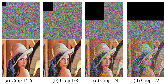
FIGURE 9. Clipped ciphertext and its decrypted image.
