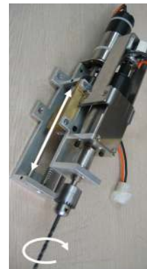
Fig. 7. The 2-DOF drill tool.
