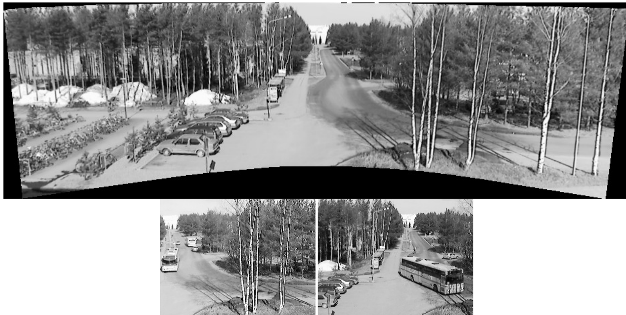
Figure 8: A mosaic ( 930 \times 291 ) constructed from a video sequence of 2000 images ( 320 \times 240 ). The sequence contains several moving objects. Two images from the sequence are shown below the mosaic. There are no moving objects present in the final mosaic because of the blending. Note: The figures are scaled for a better fit to the page.
