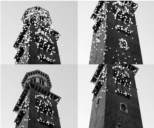
Figure 2: Upper row: the SIFT features detected from two overlapping images. Lower row: the inlier features selected by RANSAC.
