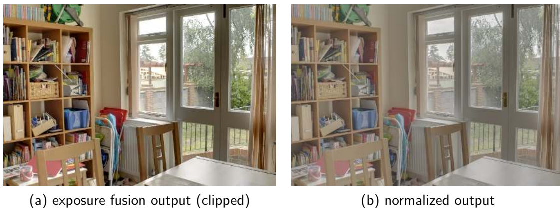
Figure 9: Result of the exposure fusion method (a) with the default parameters given in Figure 8: \omega_c = 1, \omega_s = 1, \omega_e = 1 . Saturation occurs in the bright parts of the windows, despite the fact that the input images used in these areas were not saturated. The information is preserved by the fusion but the image is clipped at the end of the process, thus incurring in information loss. In this experiment, the dynamic range of the fused image is [-0.38, 1.35] , that is, almost 1.75\times larger than the input dynamic range. For comparison, we display the linearly-compressed result on the right (b). It is not saturated, yet contrast is reduced compared to the input images of the bracketed sequence.
