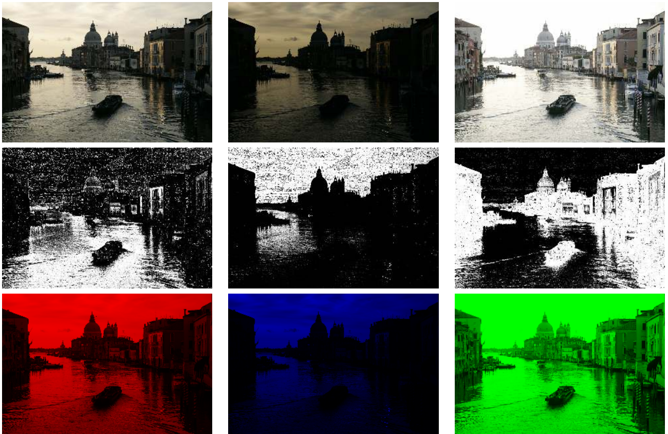
Figure 4: From top to bottom rows: Input sequence, normalized weights computed by exposure fusion, and color images that will be fused with those weights for better analysis of the merging result.
