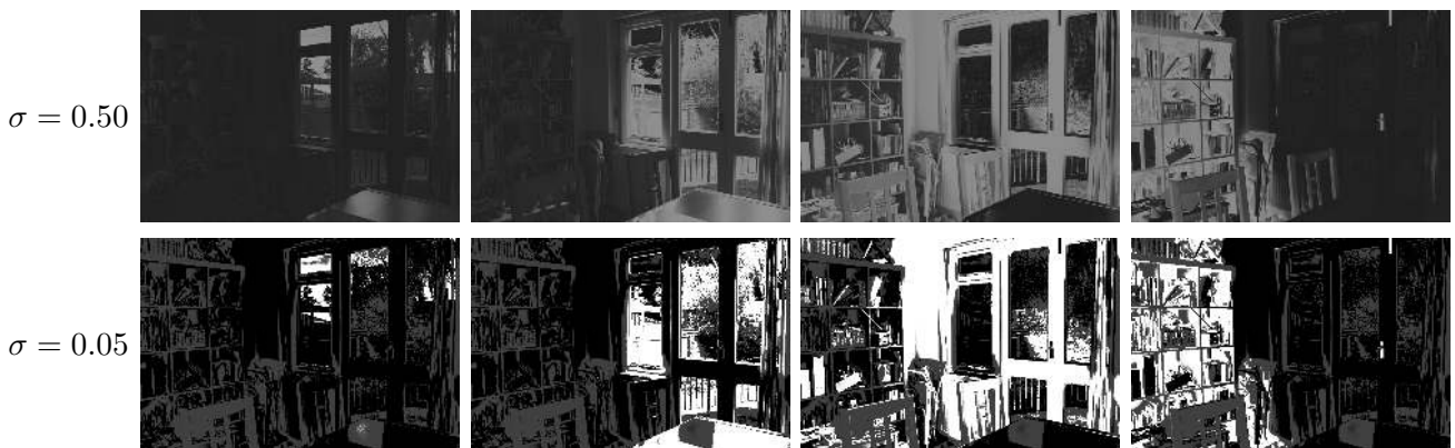
Figure 3: Weights obtained with the sequence displayed in Figure 1, with parameters \omega_c = \omega_s = 0 and \omega_e = 1 . In the top row with \sigma = 0.50 , the weights tend to be given equally in the four images. In the second row with \sigma = 0.05 , weights are given equally to all pixels whose value is far from 0.5 in every input image.
