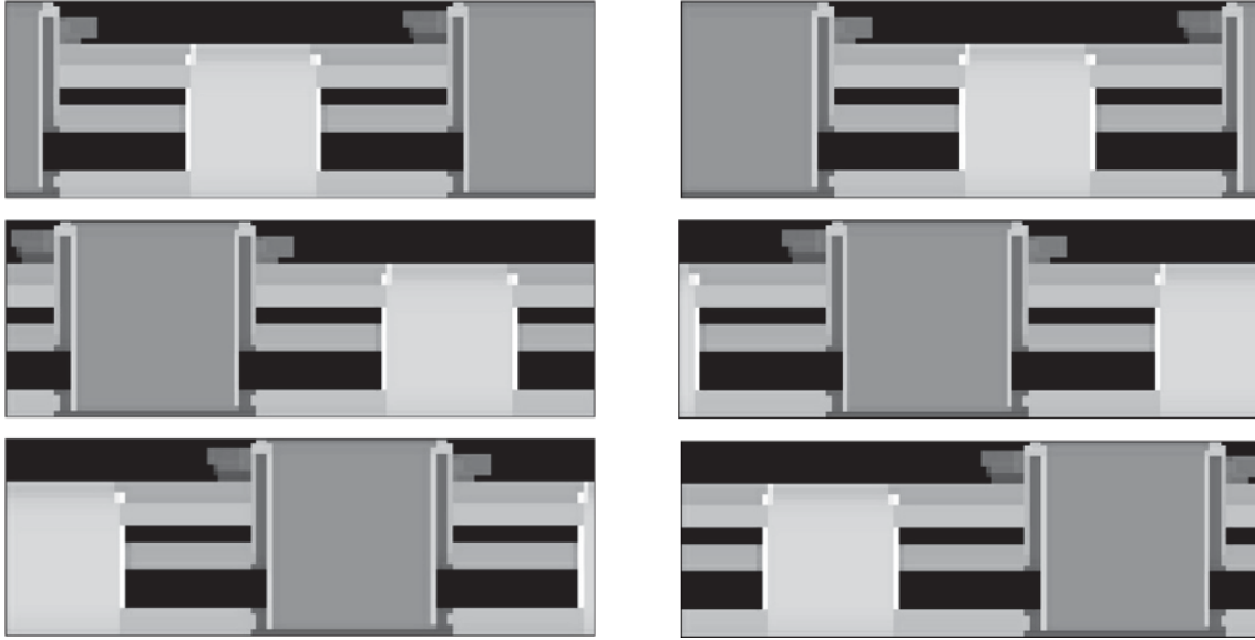
FIGURE 5: Illustration of rotation expansion. The top left image is the original view, and the others are variants, corresponding to rotation angles of 60^\circ , 120^\circ , 180^\circ , 240^\circ , and 300^\circ , read from top to bottom and left to right.
