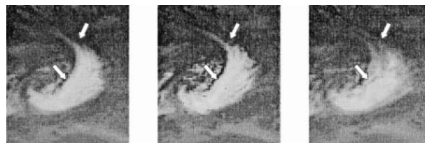
FIG. 5. Comparison of interpolated images of a Southern Hemisphere midlatitude storm using motion compensation (left) and straight temporal averaging (right). The true image is shown in the center panel. The features indicated by the arrows are discussed in the text.
