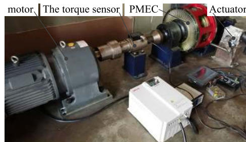
FIGURE 32. Physical diagram of the experimental platform.
