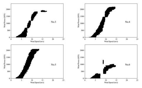
Figure 7. Abnormal data filtering result via FA.
