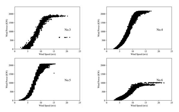
Figure 4. Abnormal data filtering result via QK.
