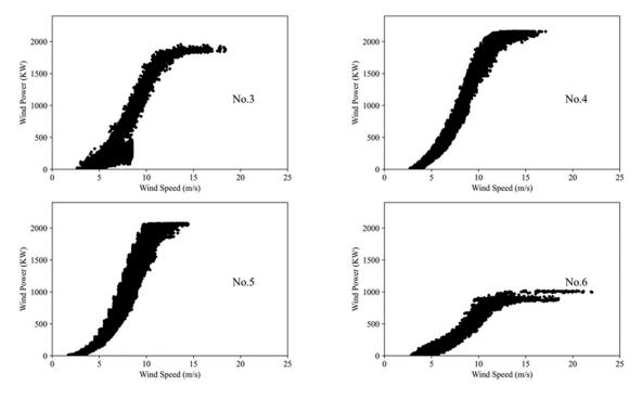
Figure 5. Abnormal data filtering result via QD.
