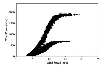
Figure 3. Abnormal data processed by I-Forest in interval detecting.
