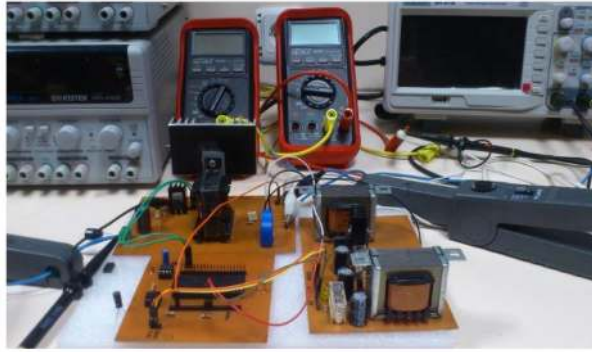
Figure 7. Photo of MPPT system.
