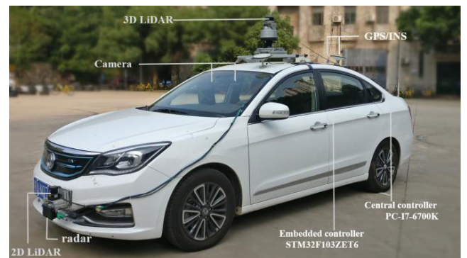
FIGURE 14. Dongfeng A60EV used for field test.
