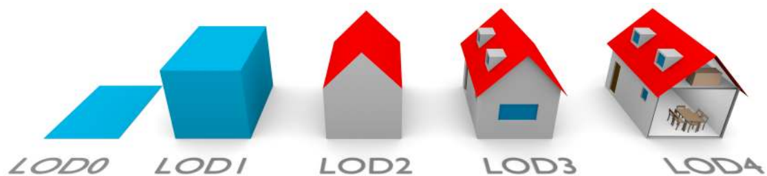
Figure 1: The five LODs of CityGML 2.0. The geometric detail and the semantic complexity increase, ending with the LOD4 containing indoor features.
