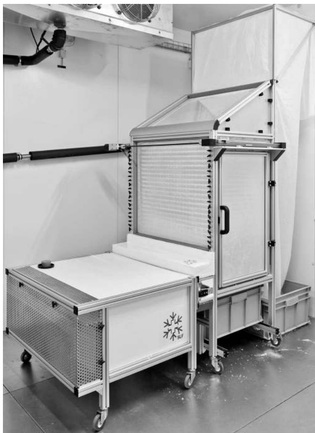
Fig. 3. Snowmaker in operation in the cold laboratory.
