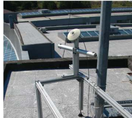
FIGURE 5: Measurement setup of incident global radiation on the platform.
