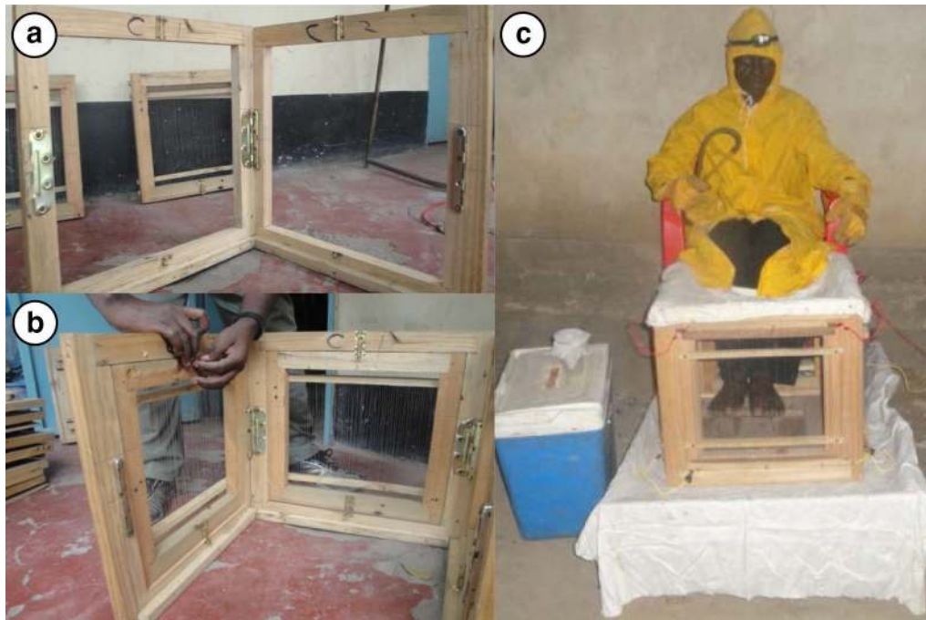
Fig. 2 Step-wise setting and improvement made to the mosquito electrocuting trap (MET). a Locking together of hinges connecting individual panels with bolts; b locking of assembled panels into the main, outer frame; c fully assembled MET in use by a human participant wearing protective clothes except for on his feet, which are placed within the MET frame
