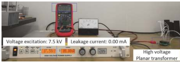
Fig. 14 Electrical insulation test
