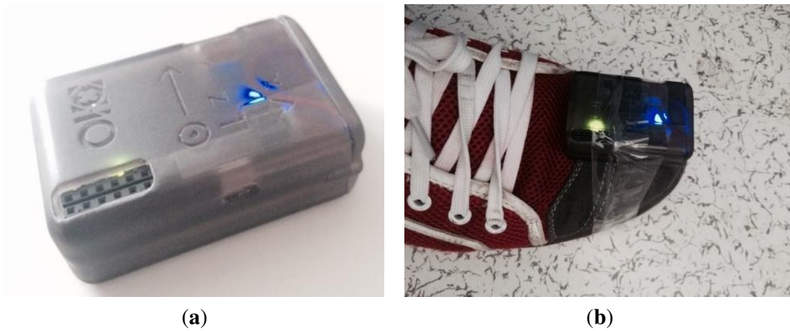
Figure 12. Photos of the equipment and their usage: (a) the x-IMU and (b) foot-mount installation.
