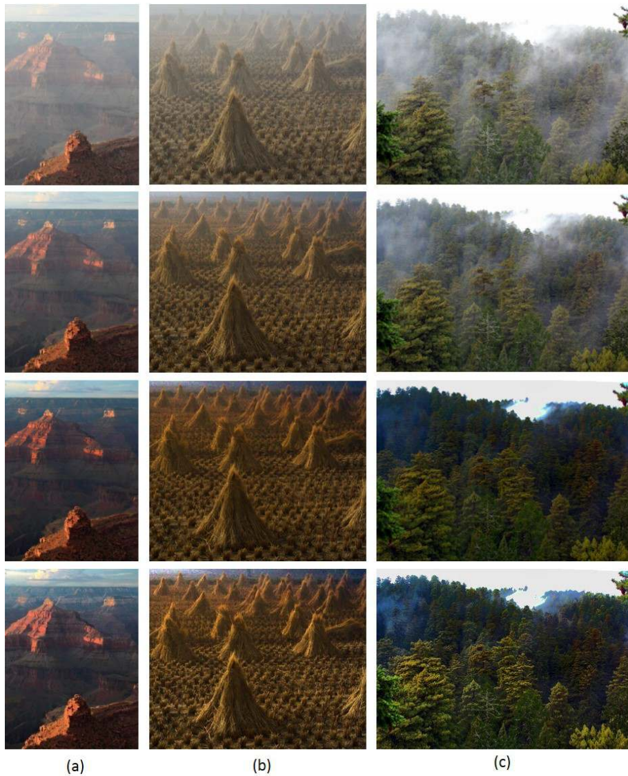
Fig. 8: Some results of our experiment. The first row is haze image. The second row is haze removal image by DCP method(parameters: (a) \omega = 0.65, n = 1 ; (b) \omega = 0.88, n = 1 ; (c) \omega = 0.83, n = 1 ). The third row is haze removal image by DCP method(parameters: (a) \omega = 0.85, n = 1 ; (b) \omega = 0.85, n = 2 ; (c) \omega = 0.83, n = 2 ). The fourth row is our result.
