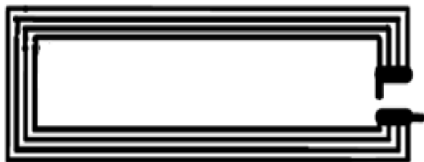
Fig. 6. 1 turn with 4 tracks
