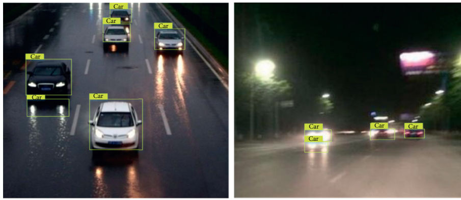
FIGURE 2: The results of car detection based on VIDAR on reflection roads.
