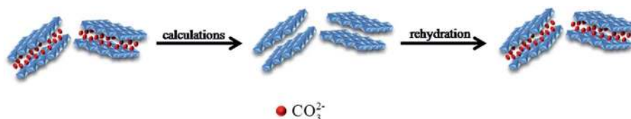
Fig. 2 The schematic representation of the Zn–Al–LDH reconstruction processes.
