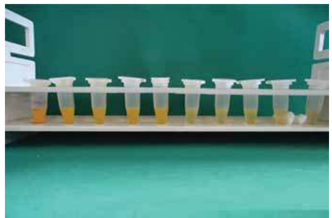
Fig. 1: Turbidity response of A. actinomycetemcomitans against serial dilutions of curcumin to check for MIC
