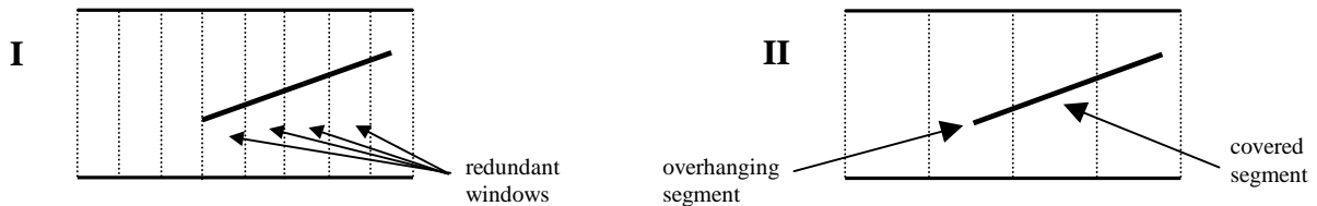
Figure 7: I) If b is too large we have the problem of redundant windows, i.e. multiple windows which could be replaced by a single window without affecting the sum \sum |R_i| . II) An illustration of the terms "overhanging segment" and "covered segment".
