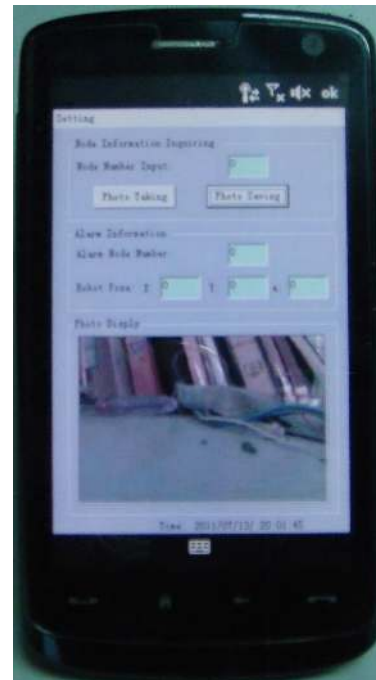
Fig. 18. Captured photo displayed on a PDA-based user interface.
