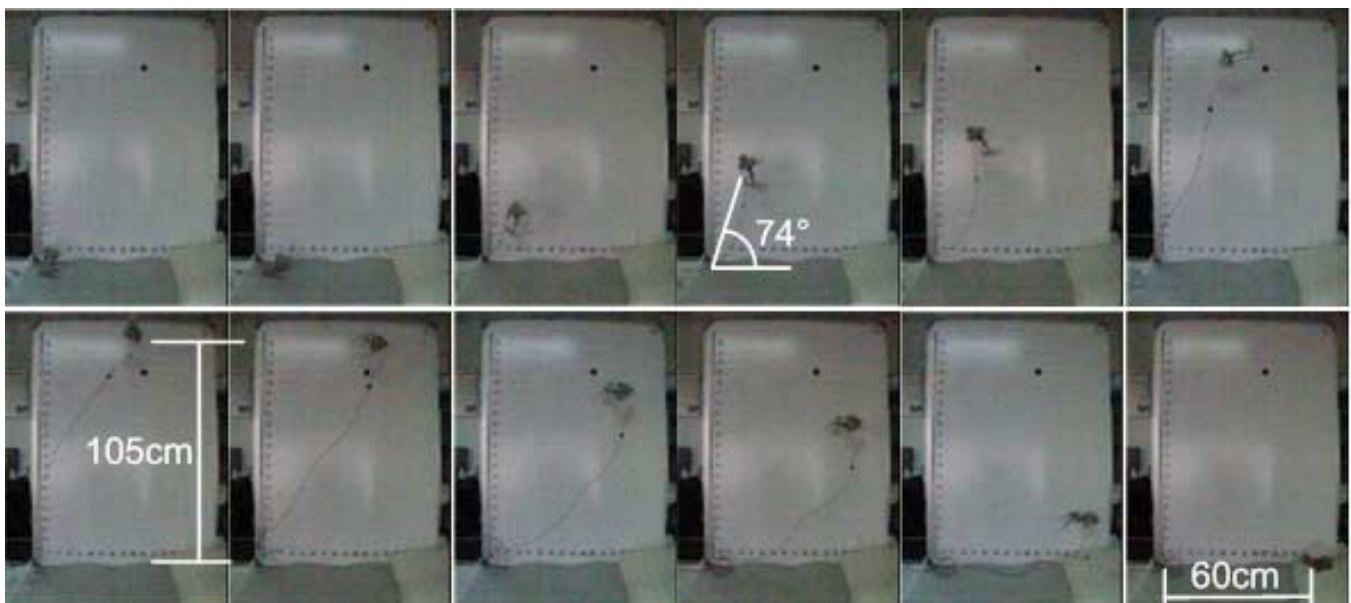
Fig. 14. Jumping sequence of the prototype robot.
