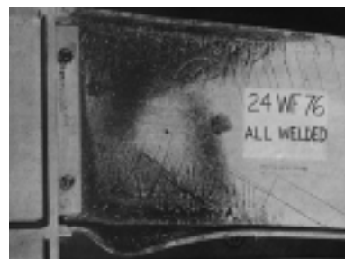
Fig. 16. Specimen of the first experiment after failure.
