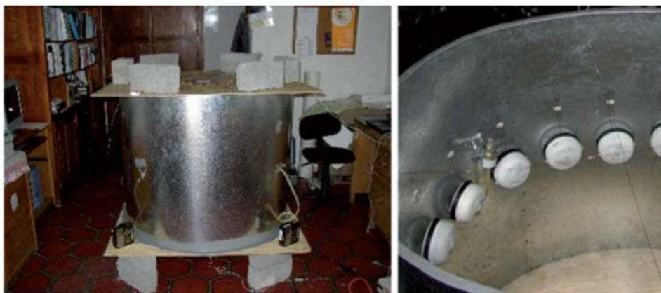
Fig. 1. Test chamber (1.2 m diameter \times 1 m height) set up in Mexican field station showing placement of UCBs and cyclone during testing.
