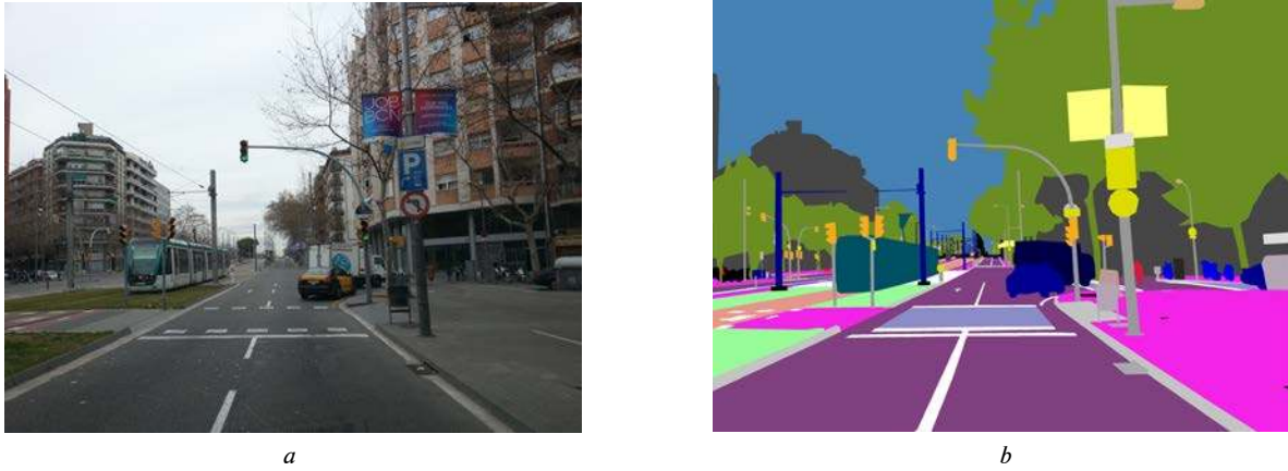
Fig. 1. A semantic image segmentation example for more than 10 classes: a – an image to be semantically segmented; b – a result of segmentation
