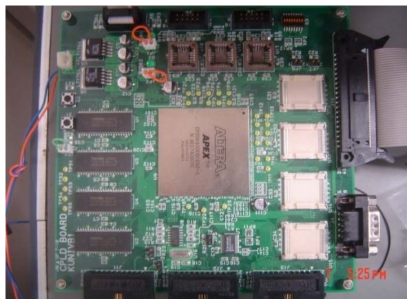
MPEG-4 SoC prototype board using an FPGA from Altera.
