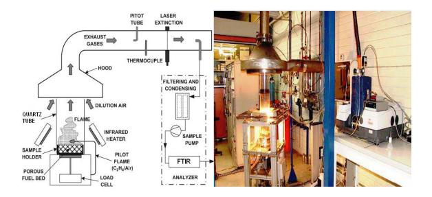
Figure 4: Modelling of generation of pollutants in an accidental fire scenario
