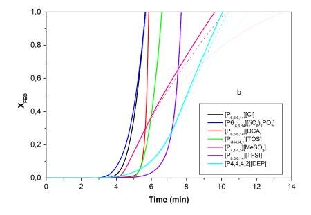
**Figure 10**: Evolution of fractional effective concentration of irritant gas involved in accidental fire scenario for a) IMBILs and b) PBILs, line for  $\tau = 3$ , dash for  $\tau = 5$  and dot for  $\tau = 10$
