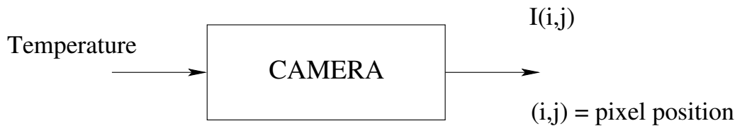
Fig. 1. From a radiometric point of view, a camera converts a temperature to a pixel gray level value I(i, j) .
