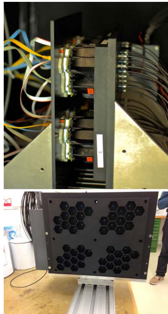
Fig. 32 Top a photo of the optical test setup with modules installed. Bottom the front panel of the setup, where the 48 illuminated optical fibers are visible
