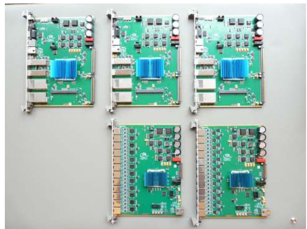
Fig. 23 Picture of three DigiCam trigger boards (top) and two digitizer boards (bottom)
