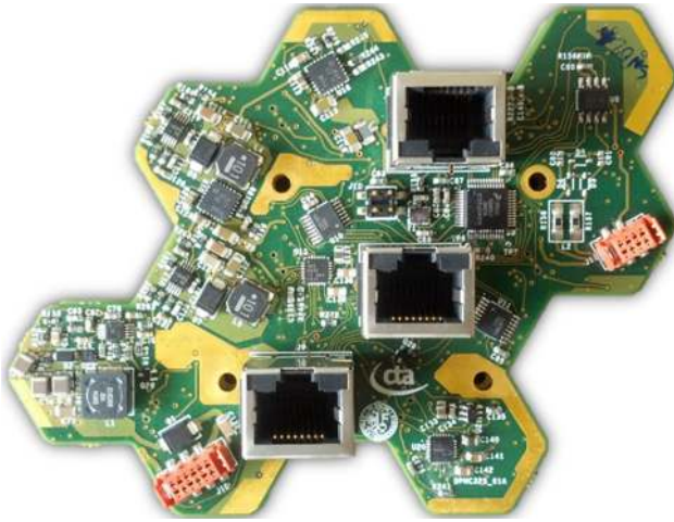
Fig. 19 A picture of the SCB from the side of the RJ45 connectors
