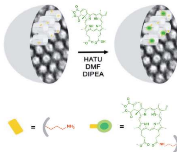
Figure 8 - Schematic representation of the synthetic procedure used to obtain Verteporfin-MSiNPs. Reproduced from (Gianotti et al. 2016) with permission of John Wiley and Sons.
