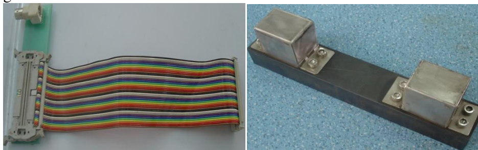
Figure 3. The transmitter coil and the magnetizer with open structure
