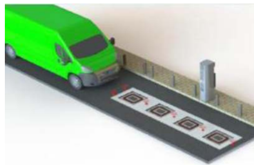
Figure 2. Fast dynamic inductive charging approach (Source: FastInCharge project)
