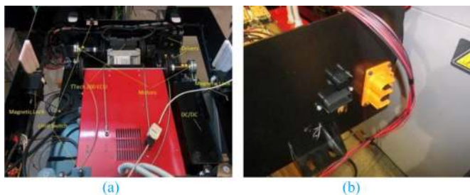
Figure 8. Black-box wires: a) Scheme of internal components wired; b) Connectors to EV (Source: FastInCharge project)
