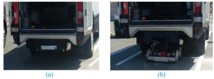
Figure 14. Positioning mechanism in the (a) up and (b) down position (Source: FastInCharge project)
