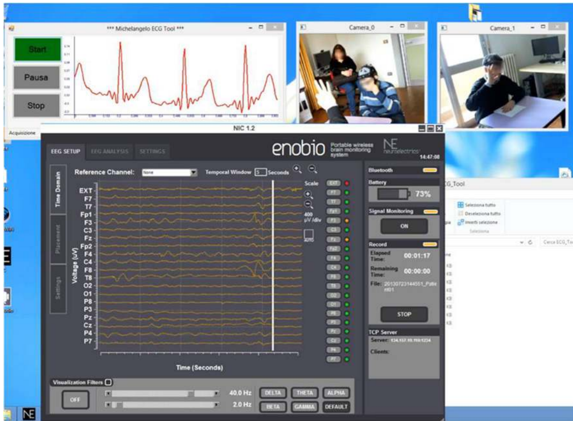
FIGURE 3 | Real-time acquisition of two camera video, ECG signal, and EEG signal during a therapeutic session.
