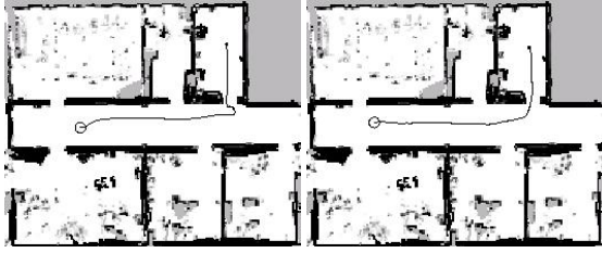
Figure 4: Typical trajectories taken by Albert when entering a room using the DWA (left) and our approach (right).
