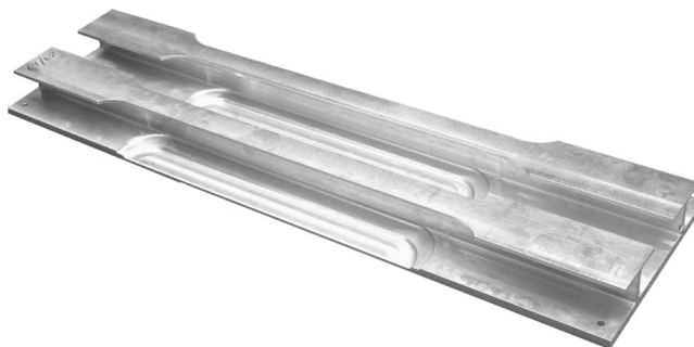
FIG. 3—As-fabricated and machined skin stringer panel.
