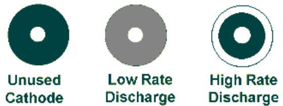
Figure 4 The "cathode freeze over" phenomenon of the Li/SOCl 2 battery
