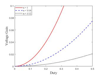
Figure 11. Ideal voltage gain of the proposed topology.
