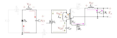
**Figure 9.** The switches  $S_3$  and  $SR_2$  are in the turned-on state.
