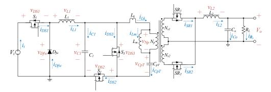
Figure 3. Equivalent circuit of the proposed IBAHB.
