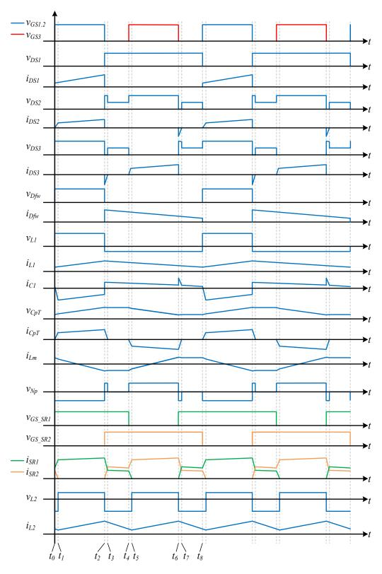
Figure 4. Transient-state waveforms of the proposed IBAHB in CCM.
