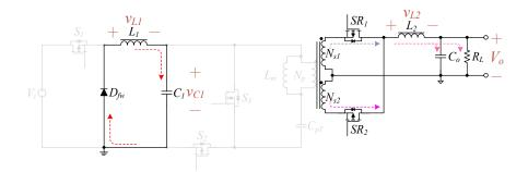
**Figure 10.** The switches  $SR_1$  and  $SR_2$  are in the turned-on state.
