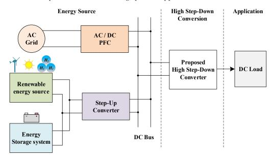
Figure 1. Block diagram of proposed high step-down converter applications.
