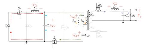
**Figure 7.** The switches  $S_1$ ,  $S_2$  and  $SR_1$  are in the turned-on state.
