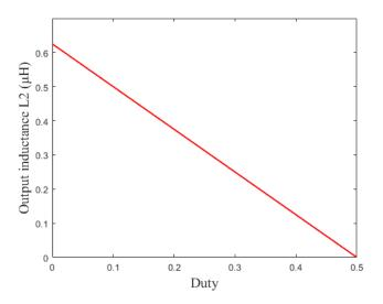
**Figure 23.** The calculated value of inductance *L*<sub>2</sub> in the boundary mode.
