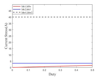
Figure 13. The estimated current stresses of switches and diode.
