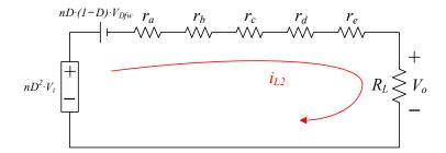
Figure 19. Simple equivalent circuit module using Equation (98).
