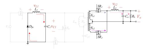
**Figure 8.** The switches  $S_1$ ,  $S_2$  and  $S_3$  are in the turned-off state.
