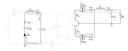
Figure 16. Equivalent circuit operating during [DT, 0.5T].
