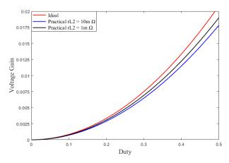
Figure 20. The calculated voltage gain of the proposed topology considering conduction loss.
