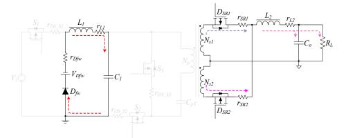
Figure 18. Equivalent circuit operating during [(0.5 + D) T, T].
