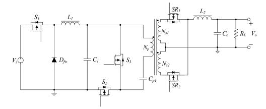
Figure 2. The topology of the proposed converter.
