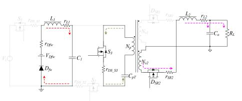
**Figure 17.** Equivalent circuit operating during [0.5T, (0.5 + D) T].
