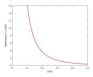
**Figure 22.** The calculated value of inductance  $L_1$  in the boundary mode.
