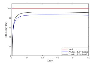
Figure 21. The calculated efficiency of the proposed topology considering conduction loss.
