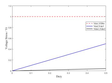
Figure 12. The estimated voltage stresses of switches.
