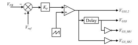
Figure 24. A diagram of the proposed control scheme.
