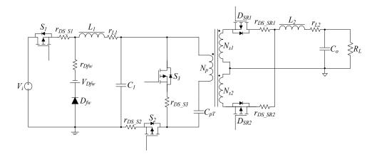
Figure 14. Equivalent circuit with parasitic components of the proposed topology.
