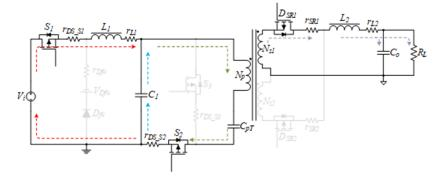
Figure 15. Equivalent circuit operating during [0, DT].
