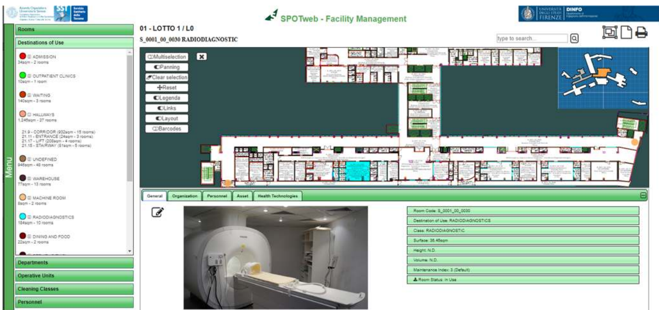
Fig. 3 Screenshot of the web-viewer. General details displayed in the bottom window. The accordion control on the left shows the functional group of the available Destinations of Use for the selected floor
