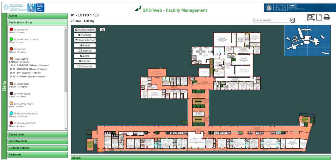
Fig. 2 Screenshot of the web-viewer. In the example all the hallways of the floor are selected (highlighted in colour)
