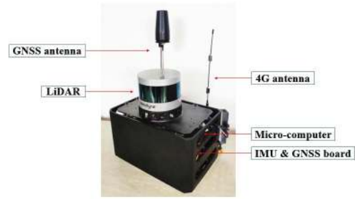
Fig. 1. Hardware composition of 3D-M-Box.
