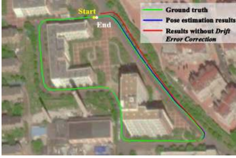
Fig. 7. Example result of drift error correction (segment #4 in Route C).
