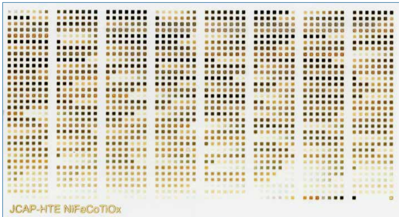
FIG. 5. High-throughput plate with a materials library consisting of quaternary metal oxides of Ni, Co, Fe, and \text{TiO}_x . Synthesis conditions: the samples were aged at 100 ^\circ\text{C} , and then calcined at 350 ^\circ\text{C} for 6-8 h in air.
