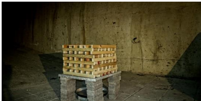
Figure 3-2 Wood crib set up
