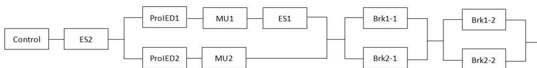
Figure 21 Alternative Transformer Bay RBD
