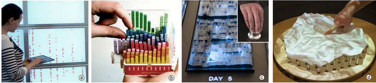
Fig. 1. Examples of beyond-desktop interactive visualizations: a) tangible range sliders for wall-sized displays [32], b) a rearrangeable physical 3D chart [33], c) an interactive data sculpture of time series [54], d) an interactive shape-changing display [40].
