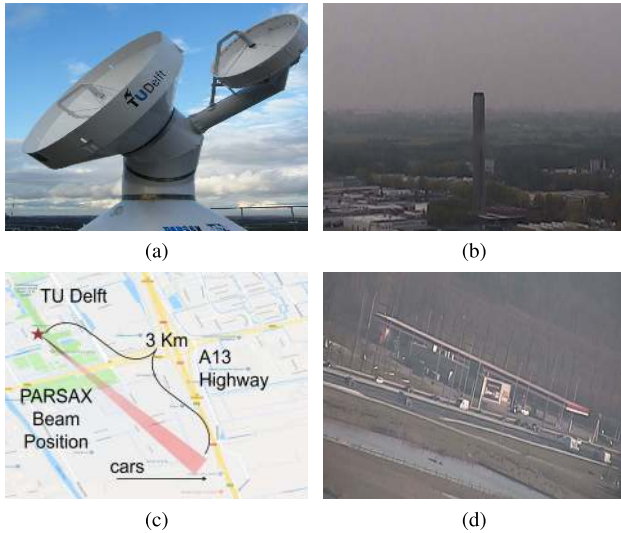
Fig. 8. Experimental setup. (a) PARSAX radar. (b) Industrial chimney as a stable-target in experiment 1. (c) Location of highway in relation to PARSAX for experiment 2. (d) Photograph of the illuminated highway area for experiment 2.
