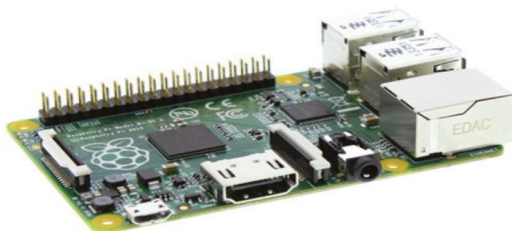
Figure 3: The Raspberry Pi 2 Model B is a credit card sized computer capable of running the Linux operating system
